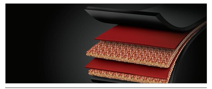
Conti<sup>®</sup>Alert is the first and only conveyor belt innovation to let you see belt wear in real time. The red bonding layer below the top cover is exposed when it's time to change the belt, creating:
